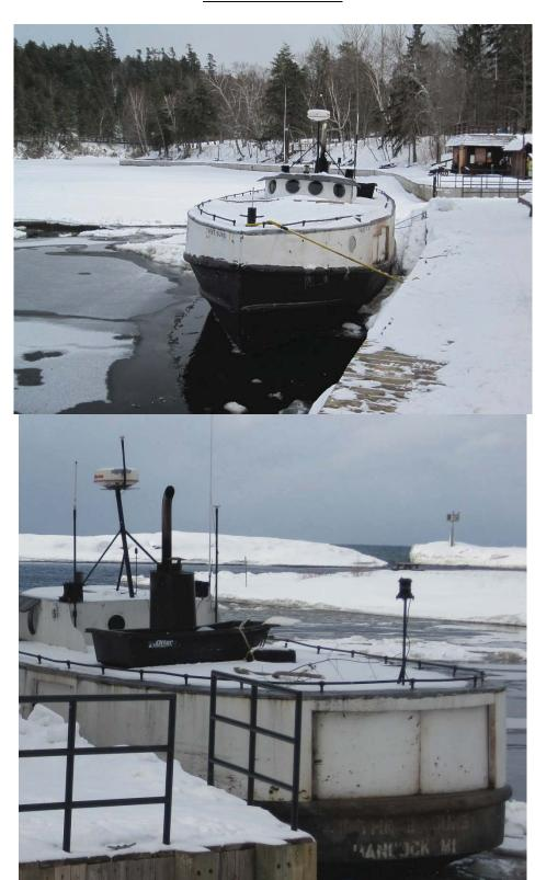
The *Three Suns* is an approximately 52 foot all-steel fish tug built in 1944 by the Burger Boat Company. The vessel, which is used by the Petersons, has a black hull and white enclosed cabin and deck. The vessel's name is visible on the starboard side near the bow of the ship and on the hull above the words "Hancock, MI" on the stern of the ship.
